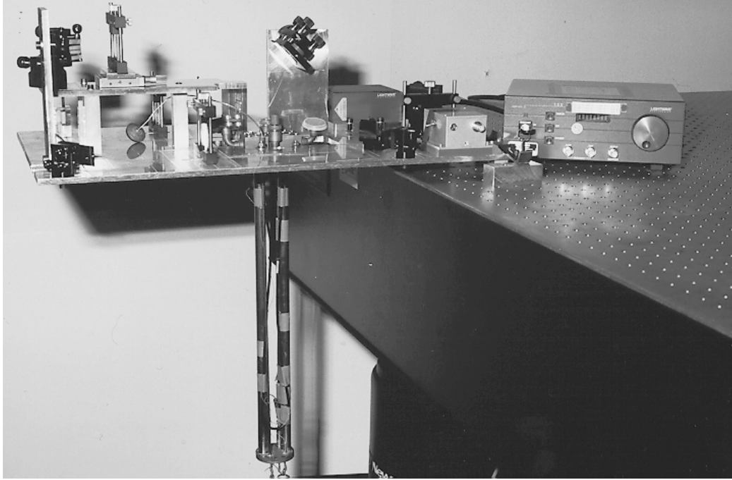
Figure 3: Experimental setup. The cryostat insert consists of a sample chamber (not shown) supported by a pair of tubes connected to a vacuum flange. The helium/nitrogen dewar (not shown) is bolted to this flange, as is the optics plate, on which the laser (at center), the focusing/alignment optics and the photodetector are mounted.
