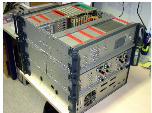
Figure E6: Right: Optics module of optical frequency comb for operation in the drop tower. It is based on an Erbium-doped fiber laser plus amplifiers. Right: electronics module. This fully phase-locked comb has first been dropped in March 2010 and has withstood 40 g acceleration upon termination of drop. Volume of optics module is ca. 30 liter.
