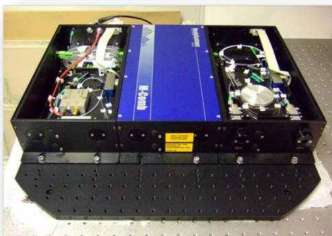
Figure E6: Right: Optics module of optical frequency comb for operation in the drop tower. It is based on an Erbium-doped fiber laser plus amplifiers. Right: electronics module. This fully phase-locked comb has first been dropped in March 2010 and has withstood 40 g acceleration upon termination of drop. Volume of optics module is ca. 30 liter.
