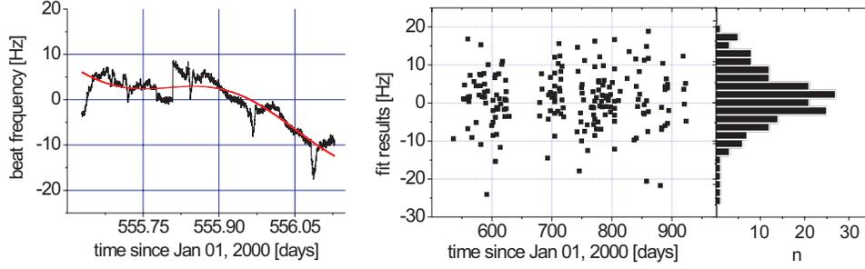
Figure 2. Left: A typical 12 h data set fitted with an offset, a linear drift, and the amplitude and phase of a hypothetical 12 h sinusoidal Lorentz violation signal predicted by the test theories. Right: Statistics over 199 such measurements.
