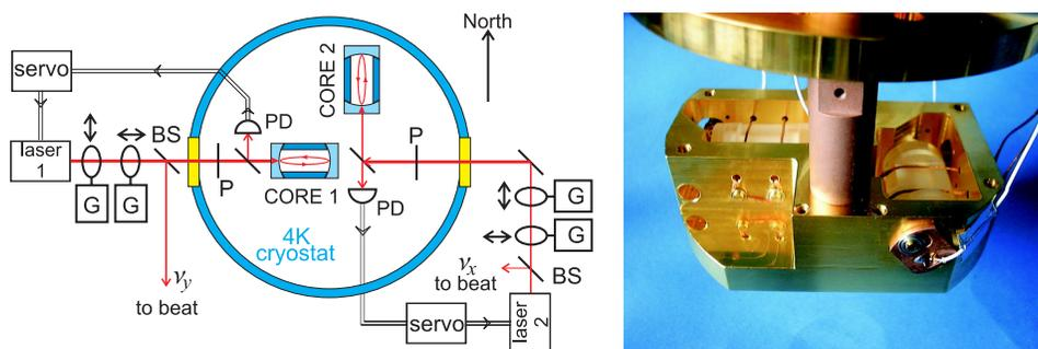
Figure 1. Schematic of the MM-experiment and photograph of the COREs inside holder.
