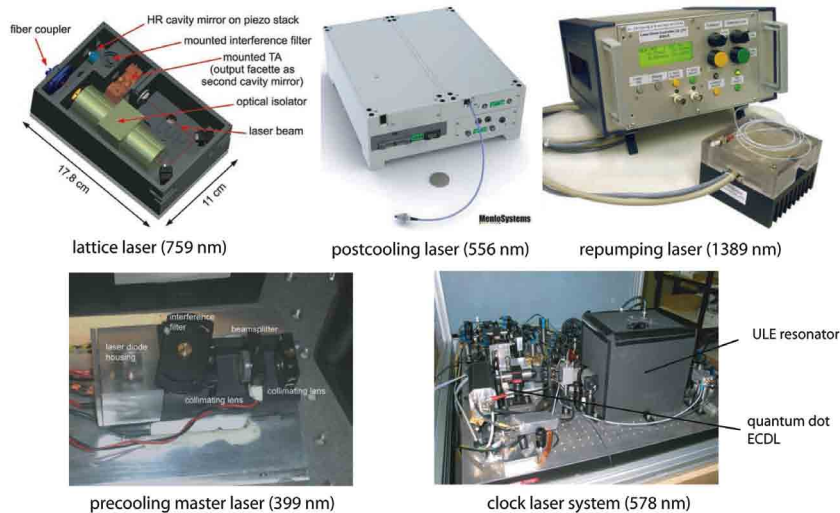
Figure 3. Overview of the laser system for the ytterbium lattice clock, comprising five lasers. Frequency stabilisation units for the first, second and fourth laser are not shown.
