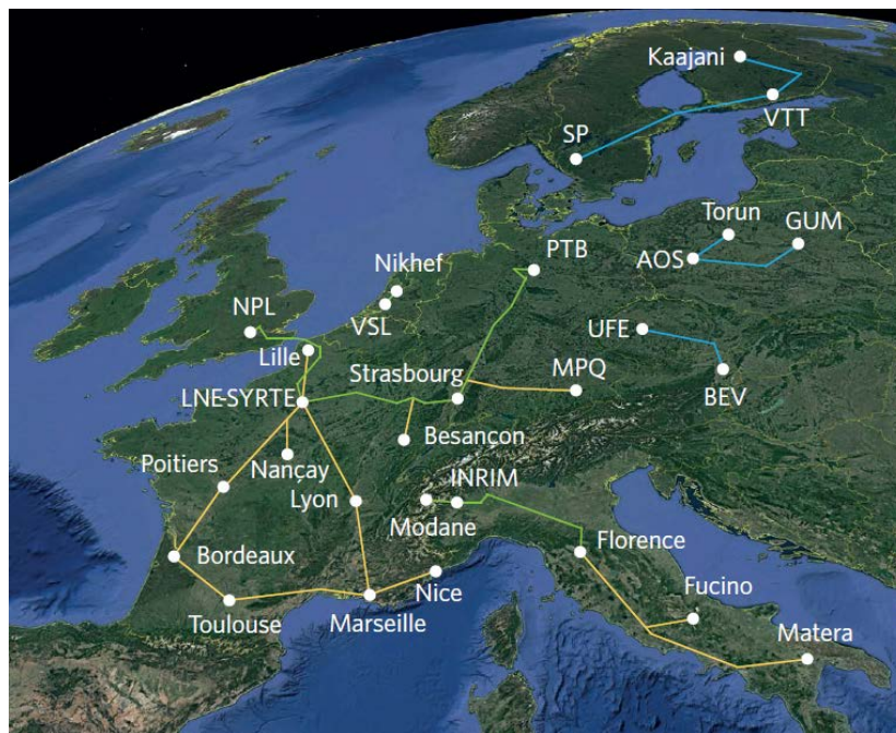
Figure 2-4 (Top) Locations with stationary high-accuracy clocks and examples of transportable optical clocks, as of 2016. (Bottom) The present and future status of fiber-optical links in Europe (from Fritz Riehle, Nature Photonics 11 , 25 (2017)): Frequency links (green), frequency links commissioned (yellow) and time links (blue). AOS, Astrogododynamic Observatory in Borowiec near Poznan, Poland; BEV, Bundesamt für Eich- und Vermessungswesen, Vienna, Austria; GUM, Główny Urząd Miar – Central Office of Measures,
