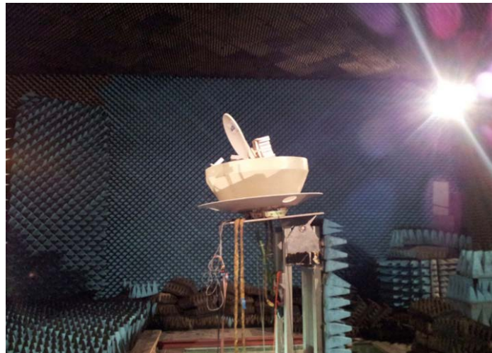
Figure A-10: ACES MWL ground terminal under test in compensated compact range facility. The I-SOC ground terminals will be based on the ACES technology.
