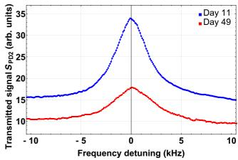
FIG. 7. Typical spectral holes observed during the long-term drift measurement. The upper blue points show a scan of a spectral hole 11 days after burning. The lower red points show another SH scanned 49 days after burning. In order to illustrate the typical deformation of the SHs, the respective frequency scales were shifted so as to center the peaks.
