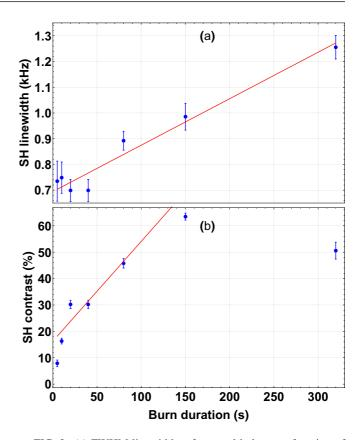
FIG. 2. (a) FWHM linewidths of spectral holes as a function of the burn time. Burn power is 1.7 nW; beam diameter is  $300 \,\mu$ m. (b) Contrast  $C_{\rm h}$  of the SHs, for different burn times.
