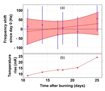
FIG. 10. (a) The change in SH frequency,  $f_{\rm shift}(t)$ , measured over a period of 14 days. All SHs were burned at time t = 0. Red line: linear fit with slope 3(7) Hz/day, or  $1.3(10) \times 10^{-19} \text{ s}^{-1}$ fractionally. The shaded region shows the  $\pm 1\sigma$  uncertainty of the fit. (b) Temperature measured at the location of the Eu<sup>3+</sup> : Y<sub>2</sub>SiO<sub>5</sub> crystal. A calibrated Cernox temperature sensor having a specified accuracy of 5 mK was used.
