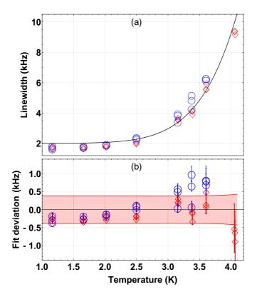
FIG. 6. Temperature dependence of the SH linewidth for rising (red diamonds) and falling (blue circles) temperature. The black line in panel (a) is a fit to the model function  $CT^7 + D$ . Panel (b) shows the deviations from the fit and the  $\pm 1\sigma$  fit uncertainty interval.
