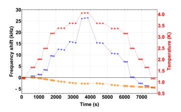
FIG. 4. Variation of the SH center frequencies as found from the AOM frequency shift  $2 \Delta f_{AOM,j}(t)$  (blue triangles) as the crystal temperature (red diamonds) is increased from 1.15 to 4 K and cooled back again. The independently occurring drift of the frequencydoubled laser frequency,  $\Delta f_0(t)$ , is shown as orange circles. Each blue point corresponds to one scan over one SH.
