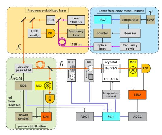
FIG. 1. Experimental setup. PD, photo detector; SHG, second harmonic generation; ULE, high-finesse ultralow thermal expansion glass optical cavity.; AOM, acusto-optic modulator; DDS, direct digital synthesizer; MC, mechanical chopper; LIA, lock-in amplifier; ATT, attenuator; SH, shutter; ADC, analog-to-digital converter; and PC, personal computer.
