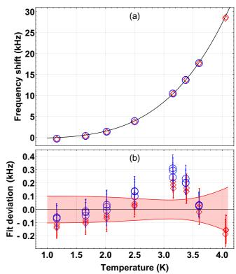
FIG. 5. Temperature dependence of the SH center frequencies for rising (red diamonds) and falling (blue circles) temperature. The black line in the upper graph is a fit to the model function  $A T^4 + B$ . Panel (b) shows the deviations from the fit and the  $\pm 1\sigma$  fit uncertainty interval.
